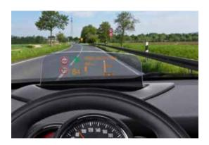
for configuration and display. Other innovations include head-up displays, which present information directly in the driver's field of vision so as to increase safety. In multimedia systems, we have offered an infotainment system with a wide range of connectivity options since 2014. The Bosch integration solution mySPIN
